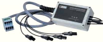
A cable with an ESSAILEC plug can be used to perform tests without disturbing or interrupting the power supply circuit on the meters and the protection relays installed in the secondary circuits of current or voltage transformers. The main advantage is that it speeds up and simplifies measurement while ensuring maximum user safety.
