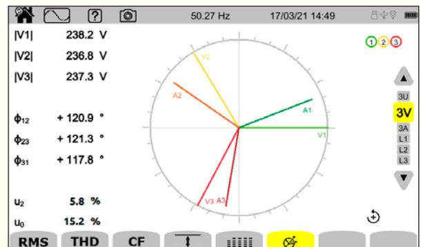
The phase relation between the voltages and currents is displayed with a vectorial diagram. The vectorial representation allows you to confirm that the instrument is connected to the mains.
